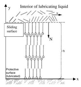
Fig. 1. Model of boundary layer: N-normal load, h-thickness of boundary layer, v-velocity of flowing of lubricating liquid
