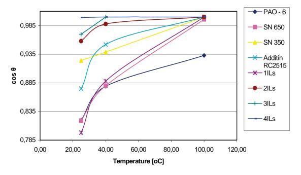
*Fig. 5. The*  $cos\theta$  *of tested lubricants versus temperature*
