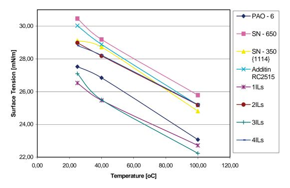
Fig .4. The surface tension of tested lubricants versus temperature
